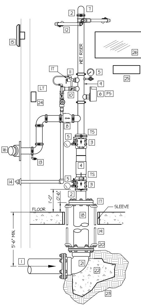
NOTE: PROVIDE SLEEVES WHERE PIPING PENETRATES BUILDING AT FLOOR AND WALLS. SEAL AROUND PENETRATION WITH FLEXIBLE MASTIC AT FLOOR. PROVIDE 2" ANNULAR SPACE
